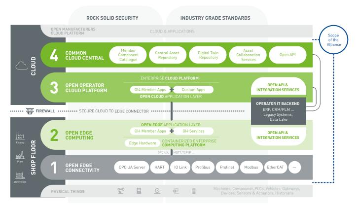
Figure 9: The Open Industry 4.0 Alliance technical architecture – a holistic IIoT framework.
