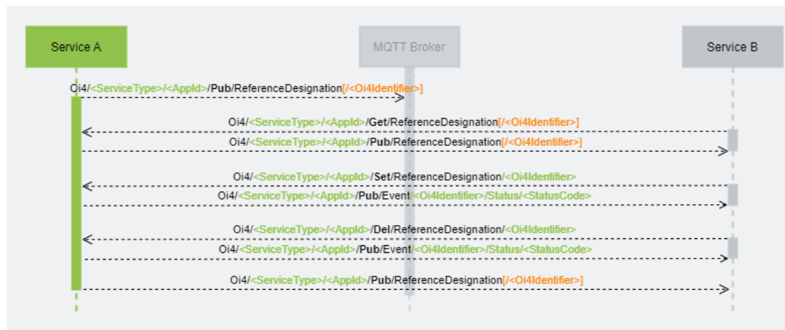
Figure 31: Sequence diagram of the interactions that can be used for the resource ReferenceDesignation
