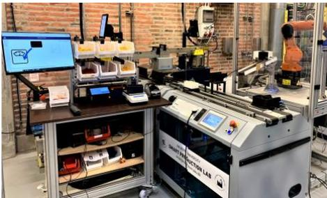
**Capture (2):** Proof of concept: Research team has connected a KUKA robot to a Microsoft Azure cloud of the LEGO Group via an edge interface of the Munich-based IoT specialist Device Insight.
